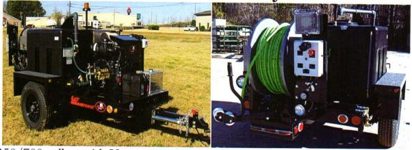
350/700 gallon with Yanmar engine and Udor pump
